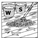
Every 3 – 4 weeks (or more frequently if required), mop your floor with a wood floor soap solution: Shake the soap bottle well before use. Pour wood floor soap into boiler-hot water using a mixing ratio of 1:40.
